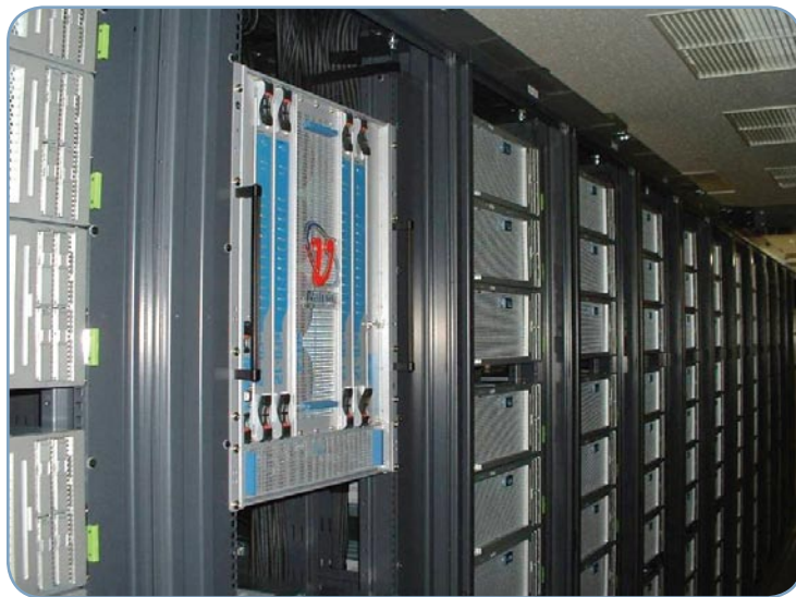
Figure 3. A scalable unit of 200 nodes powered by a Voltaire Grid Director 2012
