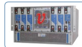
Figure 3. Voltaire Grid Director 2004 for scalable clusters ranging from 24-96 compute nodes.
