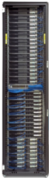
ProLiant z6000 chassis Shared infrastructure – fans, chassis, power
